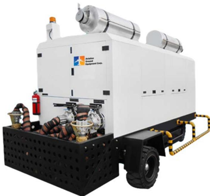
The Aviation Ground Equipment Corp. 180PPM Air Start unit will service a variety of wide-body aircraft for the commercial market. Aviation Ground Equipment Corp. proudly manufactures all of our equipment in the USA.
