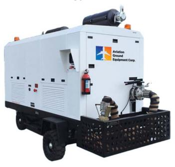
The Aviation Ground Equipment Corp. 180PPM Air Start unit will service a variety of narrow-body aircraft for the commercial market. Aviation Ground Equipment Corp. proudly manufactures all of our equipment in the USA.
